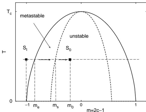
FIG. 1. Qualitative phase diagram for the Ising model. The magnetization  $m$  is related to the density  $c$  of  $C$  particles through  $m = 2c - 1$ . The solid line is the coexistence curve and the dashed one is the spinodal line.  $S_I$  is the initial state with  $m = -1$ ,  $\pm m_e$  are the equilibrium magnetizations at a given temperature  $T$ , while  $\pm m_s$  are the magnetizations at the spinodal line. The front alone would leave behind a magnetization  $m_0$ .
